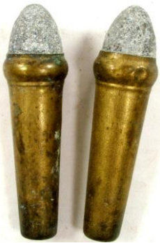
The unusual conical cartridge for the Burnside Carbine, designed by the General, which helped form a perfect seal at the breech.
