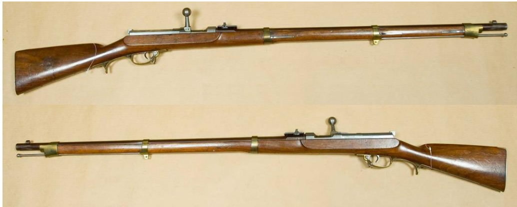
The Prussian model 1841 "Needle Gun," the first bolt rifle adopted for service
